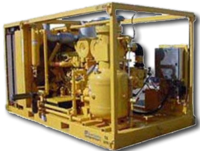
Diesel Powered Feed Air Compressor • Typical 1,600 SCFM Unit at 145 PSIG to Parker Specifications
