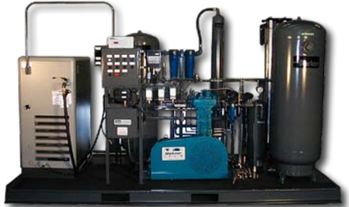
Aircraft Tire Filling Station with Gas Booster to 450 PSIG
