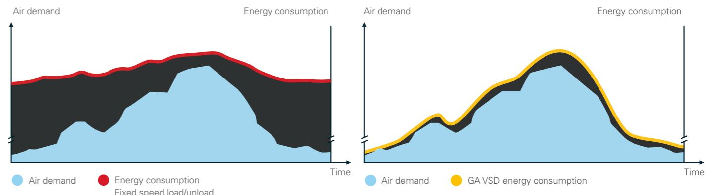
In almost every production environment, air demand fluctuates depending on different factors such as the time of the day, week or even month. Extensive measurements and studies of compressed air demand profiles show that many compressors have substantial variations in air demand. Only 8% of all installations have a more stable air demand.
