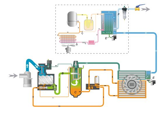
A Intake air B Air/oil mixture c 🛑 Oil
